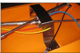
Replace ram protector bracket and insert the necessary screws.
