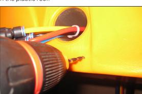
Remove bracket to drill holes with a recommended depth of 15mm.
