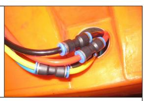
Disconnect air hoses (in roof of drafter unit) by pressing the blue ring on the end of each push-fitting then pull air tube from fitting. Note their original location for future reinstatement.
